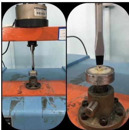
Figure 2: measure the shear bond by universal testing machine
